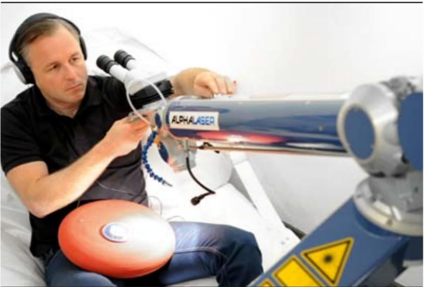
Tom Rucker working with his ALM 200, a state-of-the-art laser welding machine originally designed for industrial applications by Munich based company ALPHA LASER GmbH
